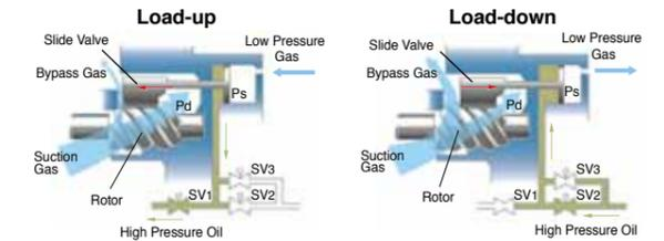
Pd: Discharge pressure, Ps: Suction pressure, SV1,2,3 : Solenoid valve : Valve open : Valve close
